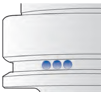
Fine-balanced with balancing bores in the flange
